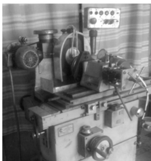
Fig. 7. LPG scheme: 1 – grinding wheel 2 – cassette with parts 3 – laboratory unit for LPG
