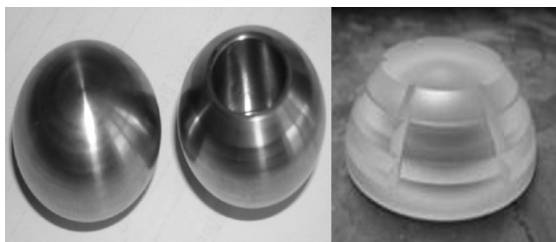
Fig. 6. Samples of the titanium head and sapphire cup for endoprosthesis of hip joint
