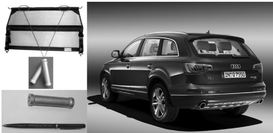
Figure 2. Aluminium foam crash energy absorber mounted into the dividing net of Audi Q7.
